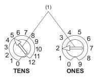
(1) Insert a screwdriver here to set the address
